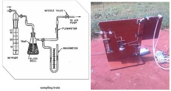
Figure no 1: Set up of the Air sampling train
